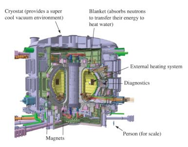
*Note.* This figure denotes the inner model of ITER fusion reactor (Faizan, 2019).
